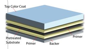
A two coat system with a Primer and Color Top Coat to
